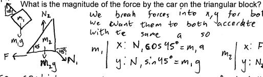
We break forces into x, y for both blocks, but we want them to both accerdite in the -x direction with the same a so
