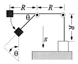
The left mass is released from rest. At what angle  $\theta$  will the right mass just begin to lift off the table?
